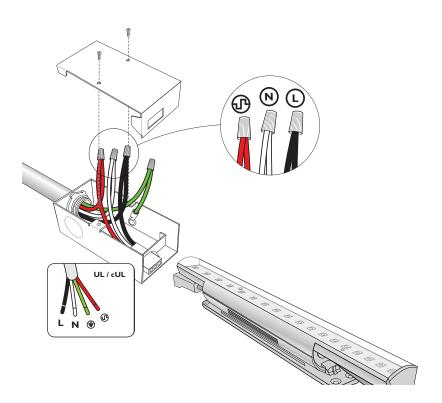
7. Secure connections within the Data Enabler Pro housing.
