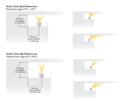
These diagrams provide general guidelines for positioning iColor Cove QLX Powercore fixtures in coves with matte white surfaces. Specific dimensions and positioning depend on the details of your installation.
