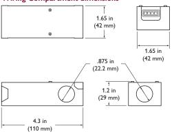
So If using the Wiring Compartment to run conduit from Data Enabler Pro to the first fixture in a run, make sure you leave enough space at the end of the run to accommodate the Wiring Compartment.
