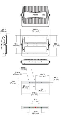
Universal power input range — eColor Reach Powercore gen2 accepts a universal power input range of 100 – 240 VAC, allowing consistent installation around the world.
