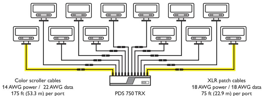
The number of ColorBlast TRX fixtures that each power / data supply can support is determined by the such factors as the supply's capacity and number of available ports. The PDS-750 TRX, for example, offers power / data ports for connecting up to 12 ColorBlast TRX fixtures simultaneously.
