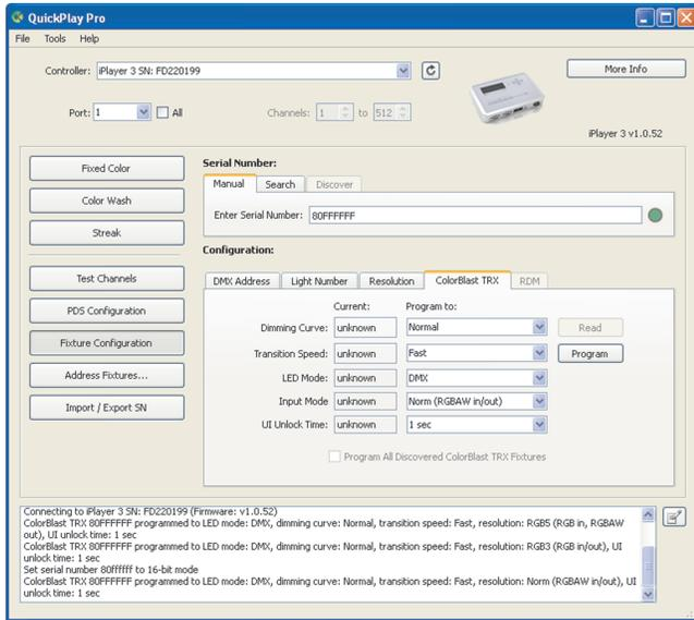
4. To set the fixture's starting DMX address, click the DMX Address tab, enter a starting DMX address in the New DMX Address box, and click Program.
