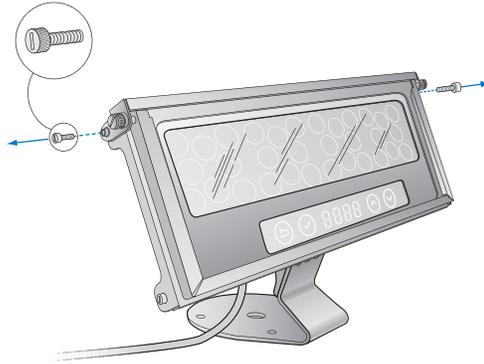
2. Grab the tabs at the top of the lens bezel and gently flex it apart until the tabs release from the fixture housing. Pivot the bezel and accessory holder forward to access the lens.
