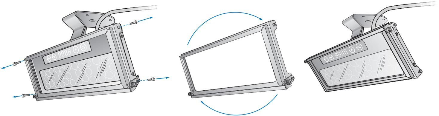
2. Loosen the two captive thumbscrews located on the upper edge of the accessory holder, and pivot the top of the accessory holder back to expose the slot.
