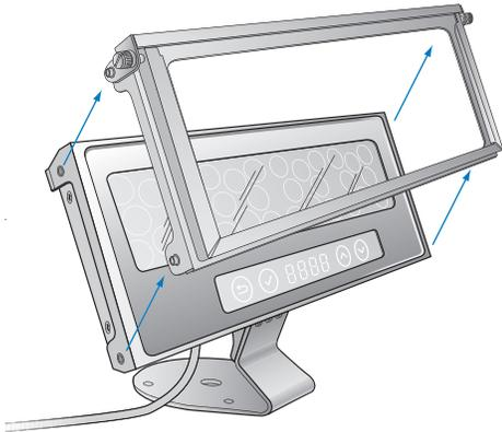
3. Secure the lens bezel directly to the fixture housing using the four included 6-32 Phillips head stainless steel screws.
