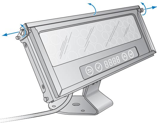
3. Slip the spread lens or accessory into the accessory holder slot.
